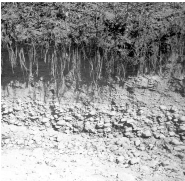
Figure 15. Exposed underlying sand and gravel deposits are typical of alluvial soils, such as Ross and Medway.
